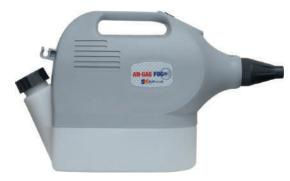
ULV nebulizer (5 to 20 microns) compact and easy to use. The powerful engine generates a stream of air that carries micronized droplets in suspension. By rotating the front nozzle it is possible to adjust the flow rate and the size of the drops emitted. The base allows a stable position thanks to the low center of gravity.
