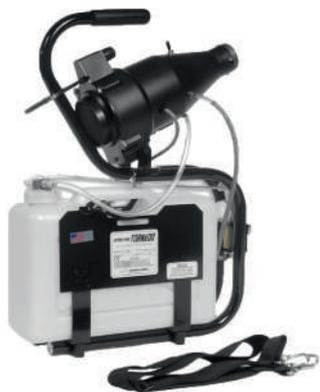
Ideal for moistening treatments in greenhouses and nurseries, for disinfection and for the supply of disinfectants and germicides. Production of droplets from 10 to 40 microns. Equipped with a removable tank for the product, filter and precision dispense valve that allows you to adjust the consumption up to 26 l/h.
