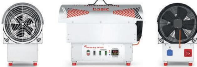
Easy to use and lightweight heat generator (only 19 kg). Update 3.0 improved performance in terms of maximum achievable temperature (up to 70 °C) and safety, with the use of additional sensors on fan operation and shutdown in case of overheating. The installed test button verifies that all the equipment works correctly before starting the treatment.
